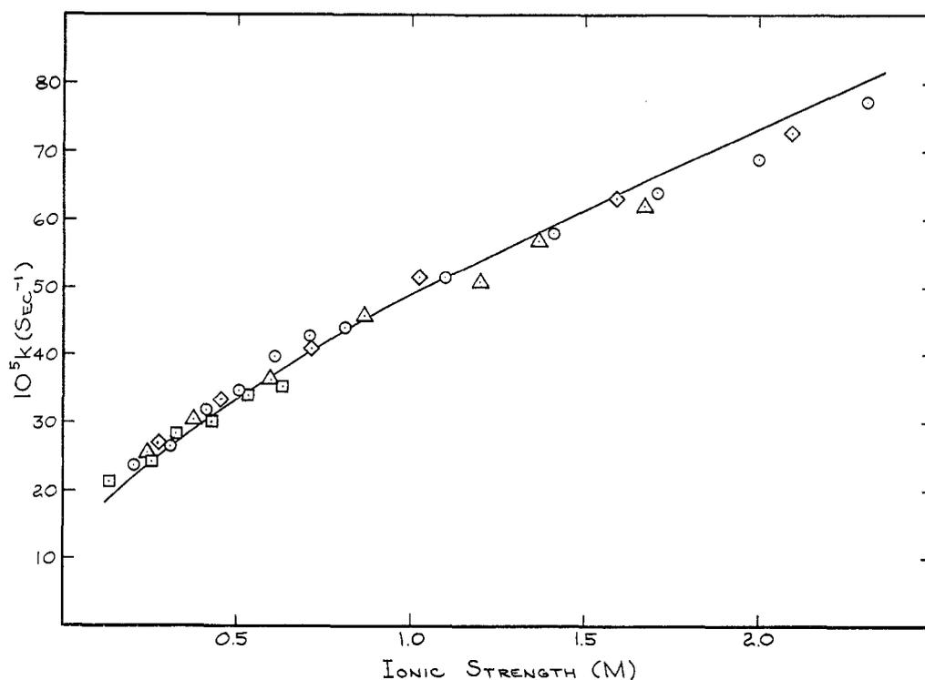
Figure 5.—Variation of anation rate constant with ionic strength using different salts; (complex ion) =  $10^{-2} M$ ; (oxalate) =  $0.1 M$ ;  $\circ$ ,  $KNO_3$ ;  $\Delta$ ,  $LiNO_3$ ;  $\diamond$ ,  $NaNO_3$ ;  $\square$ ,  $NaClO_4$ .
