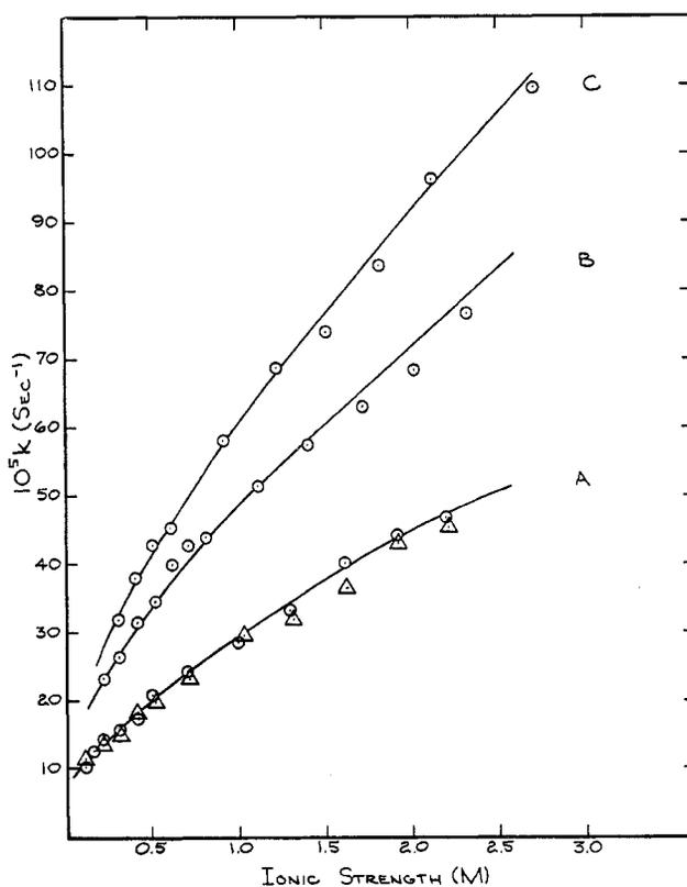
Figure 4.—Variation of anation rate constant with ionic strength and acidity; (complex ion) =  $10^{-2} M$ . A: ○,  $(H_2C_2O_4) = (HC_2O_4^-) = 0.1 M$ ; pH  $\sim 1.3$ . A: △,  $(HC_2O_4^-) = 0.1 M$ ; pH  $\sim 2.7$ . B:  $(HC_2O_4^-) = (C_2O_4^{2-}) = 0.05 M$ ; pH  $\sim 4.3$ . C:  $(C_2O_4^{2-}) = 0.1 M$ ; pH  $\sim 6.0$ .
