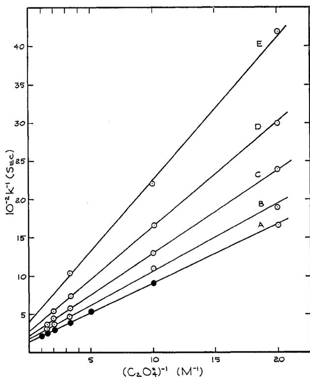
Figure 3.—Inverse relationship between observed anation rate constant and oxalate concentration; (complex ion) =  $10^{-2} M$ ; pH  $\sim 6.0$ ; ●, observed points; ○, points interpolated from Figure 2. Ionic strengths ( $M$ ): A, 2.7; B, 2.0; C, 1.5; D, 1.0; E, 0.5.
