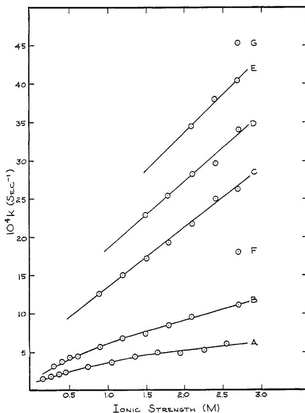
Figure 2.—Variation of anation rate constant with ionic strength at various oxalate concentrations; (complex ion) =  $10^{-2} M$ ; pH  $\sim 6.0$ ; (oxalate): A, 0.05 M; B, 0.10 M; C, 0.30 M; D, 0.50 M; E, 0.70 M; F, 0.20 M; G, 0.90 M.
